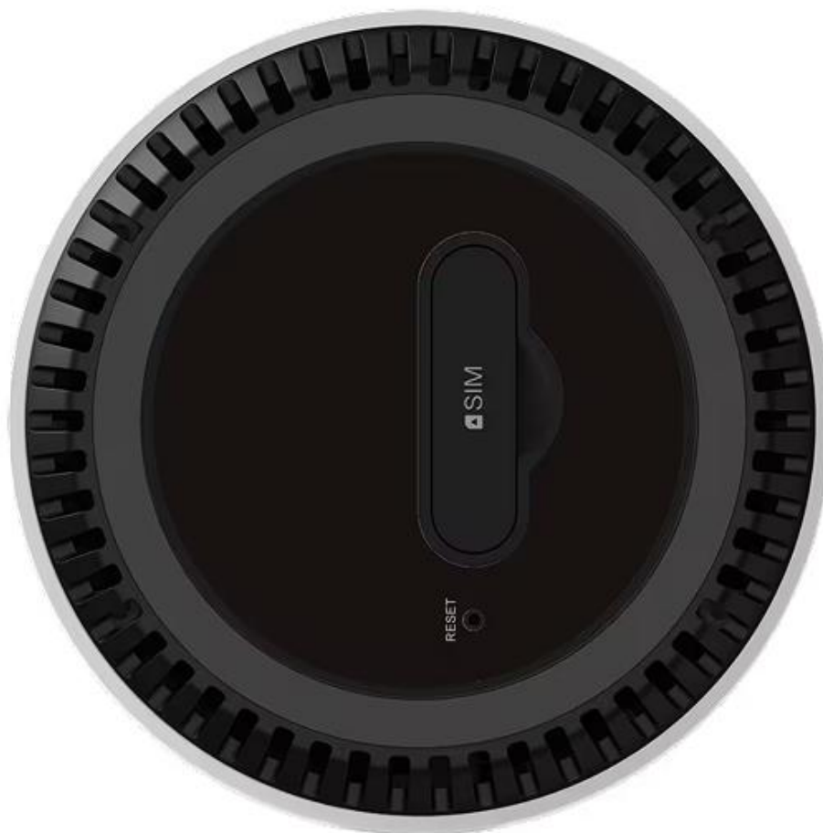
Fig. 4 — Bottom: nano SIM slot and Reset button
